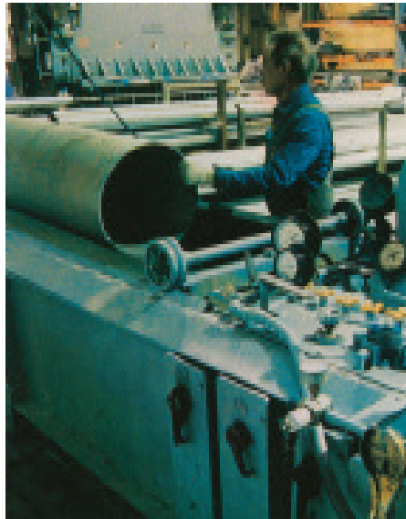
Hydrotesting verifies pressure capabilities of pipe and tubing.
