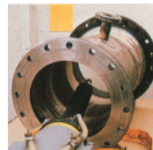
Radiographic inspection checks the integrity of welds.
