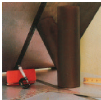
Geometric accuracy is checked on all Alaskan fittings.
