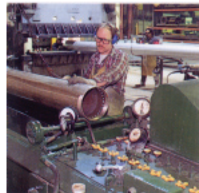
Hydrotesting testing checks for leaks and structural integrity.
