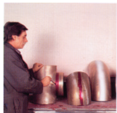
Liquid penetrant examination locates surface defects which may be too small to see visually.
