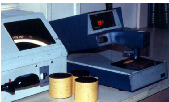
A specialized film reader and digital densitometer are used in interpreting radiographic film.
