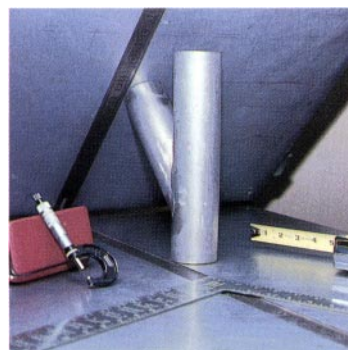
Angle standard being used to check the geometric accuracy of prefabricated piping items.
