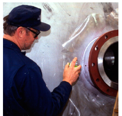
Liquid penetrant examination locates hidden surface defects which may be too small to see visually.
