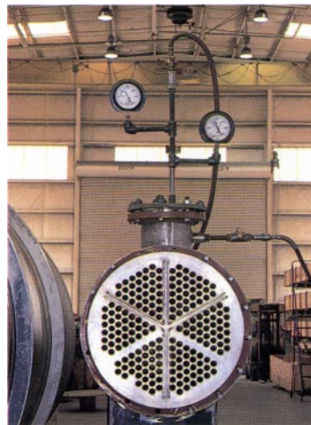
Hydrostatic testing checks for leaks and structural integrity.
