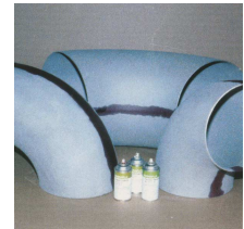
Liquid penetrant examination locates hidden surface defects.
