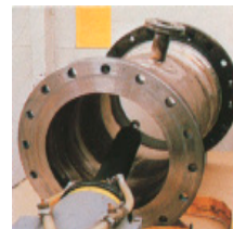
Radiographic inspection checks the integrity of welds.
