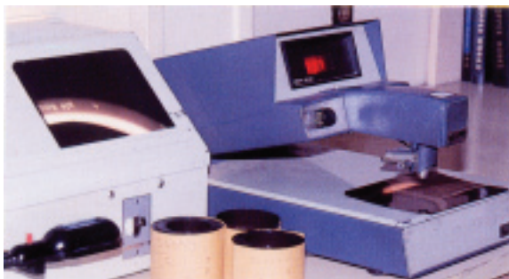
A specialized film reader and digital densitometer are used in interpreting radiographic film.
