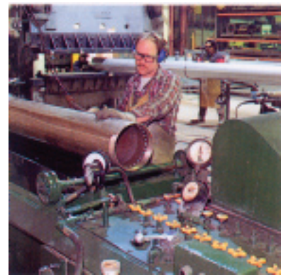
Hydrotesting testing checks for leaks and structural integrity.
