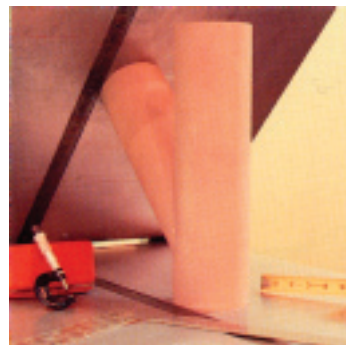
Angle standard being used to check the dimensional requirements of prefabricated piping items.
