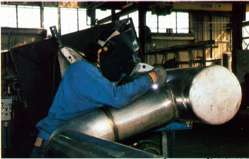
A welder attaching a piping section to a smooth-drawn tee outlet—a special feature of Alaskan prefabricated piping.
