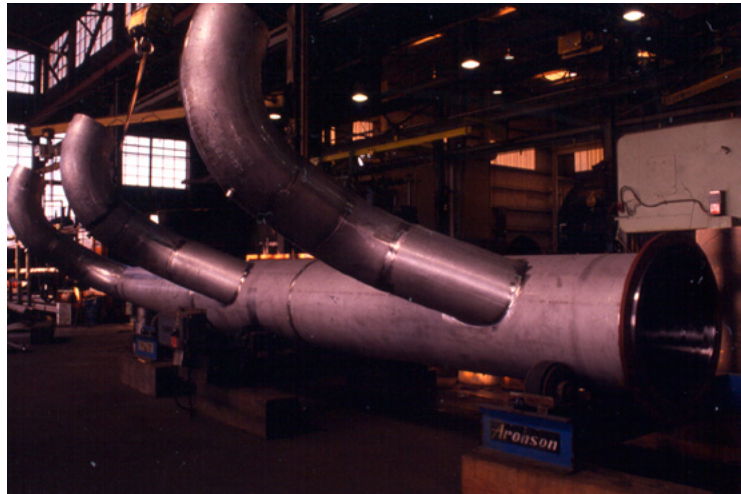
Piping header with polished internal surfaces.
