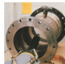
Radiographic inspection checks the integrity of welds.
